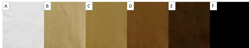
Fig. 1- photograph of: (A): as-electrospun and stabilized fibers at (B) 230 °C, (C) 240 °C, (D) 250 °C, (E) 280 °C and (F) CNF.
