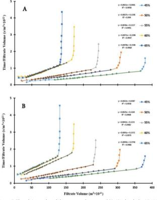
Figure 7. Plot of t/v vs v for solid percent in the range of 45-65% for cloths A7 (A) and A12 (B), (pressure: 0.6 bar, cake thickness: 13 mm, time: 10 min).
