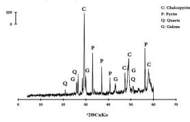
Figure 2. X-ray diffractogram (XRD) of the concentrate sample from the Qaleh Zari copper mine.
