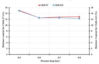
Figure 11. Effect of pressure drop on cake moisture content, (cloths: A7 and A12, solid percent: 55% (A7) and 50% (A12), cake thickness: 13 mm, time: 10 min).
