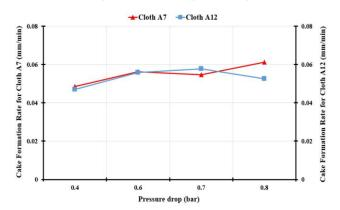
Figure 9. Effect of pressure drop on cake formation rate, (cloths: A7 and A12, solid percent: 55% (A7) and 50% (A12), cake thickness: 13 mm, time: 10 min).
