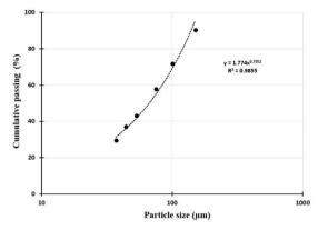
Figure 3. Particle size distribution of the representative sample of copper concentrate.
