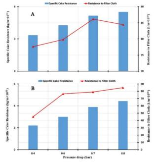
Figure 10. Effect of pressure drop on specific cake resistance and resistance to filter cloth, (cloths: A7 (A) and A12 (B), solid percent: 55% (A7) and 50% (A12), cake thickness: 13 mm. time: 10 min).
