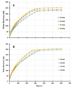
Figure 12. Effect of pressure drop on water recovery versus time, (cloths: A7 (A) and A12 (B), solid percent: 55% (A7) and 50% (A12), cake thickness: 13 mm, time: 10 min).
