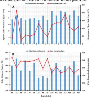
Figure 6. The effect of cloth type on the specific cake resistance and resistance to filter cloth (A) and cake moisture content and cake formation rate (B), (pressure drop: 0.6 bar, cake thickness: 13 mm, solid percent: 60% w/w, time: 10 min).
