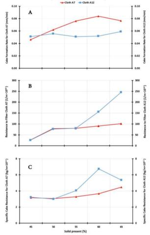
Figure 8. Effect of solid percent on cake formation rate (A), resistance to filter cloth (B) and specific cake resistance (C); (cloths A7 and A12, pressure drop: 0.6 bar, cake thickness: 13 mm, time: 10 min).
