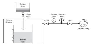
Figure 4. Operational apparatus of filtration process in Lab.
