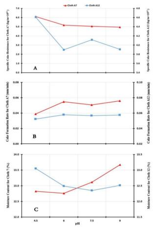
Figure 14. Effect of pH changes on specific cake resistance (A), cake formation rate (B), and cake moisture content (C); (cloths: A7 and A12, pressure drop: 0.6 bar, cake thickness: 13 mm, time: 10 min).
