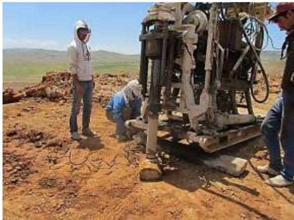
**Fig 4.** Drilling of in the tailings and natural substrate of Site 1 with a skate drill D750
