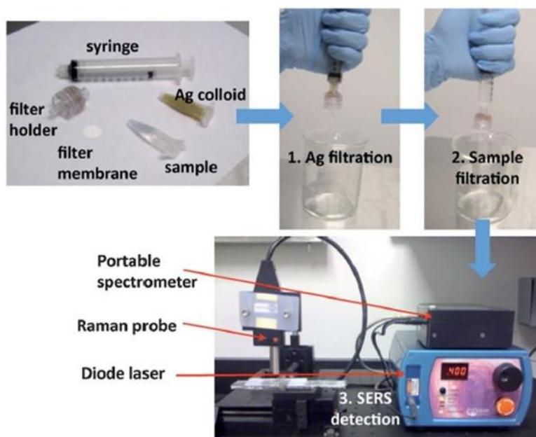
**Figure 1.** Preparation of SERS-active substrates using syringes by passing a silver nanoparticle solution through a filter membrane. Reprinted from *Analyst*, Volume 137, Issue 5, Pages 1168-1173, Yu, Wei W. and White, Ian M., A simple filter-based approach to surface enhanced Raman spectroscopy for trace chemical detection, Copyright 2012, with permission from The Royal Society of Chemistry [20].
