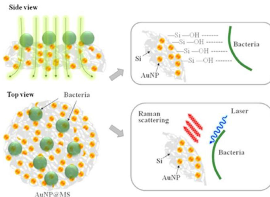
**Figure 3.** Schematic of a SERS substrate and bacteria [56].
