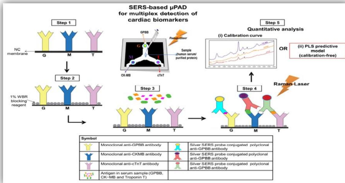
**Figure 6. Schematic of multiplex SERS detection of cardiac biomarkers at respective reaction zone(s), G for GPBB, M for CK-MB, and T for cTnT on  $\mu$ PAD [77].**
