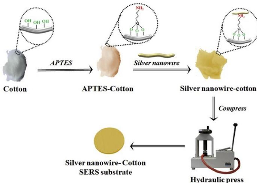
**Figure 2.** Schematic of cotton fiber membrane-silver nanowires deposited on paper as a SERS biosensor presented by Ankudze et al. [53].
