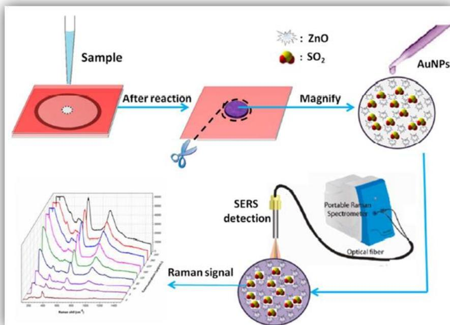
**Figure 5. Illustration of  $\mu$ PAD-SERS for on-site detection of sulphite in wines. Reprinted from Analyst, Volume 141, Issue 19, Pages 5511-5519, Chen, Miao and Yang, Hua and Rong, Liya and Chen, Xiaoqing, A gas-diffusion microfluidic paper-based analytical device ( $\mu$ PAD) coupled with portable surface-enhanced Raman scattering (SERS): facile determination of sulphite in wines, Copyright 2016, with permission from The Royal Society of Chemistry [73].**
