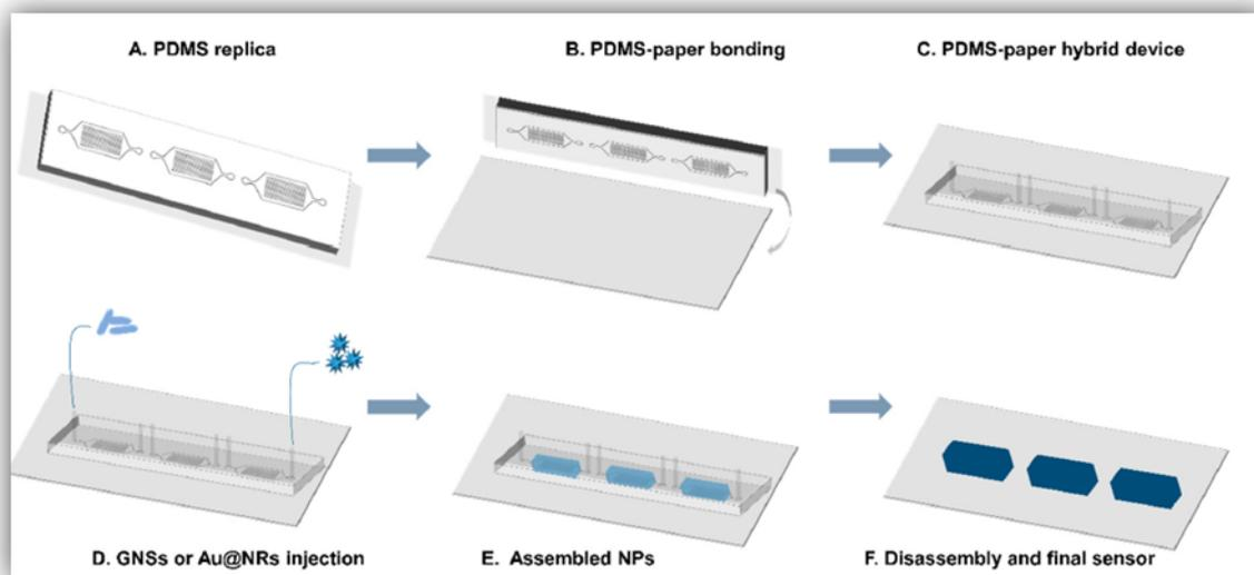
**Figure 8. Schematic of the preparation of the hybrid PDMS-paper device (A–C) injection and self-assembly of the nanoparticles (D) Raman model molecule or lysed cells injection (E) final disassembly of the paper sensor for analysis (F) [72].**
