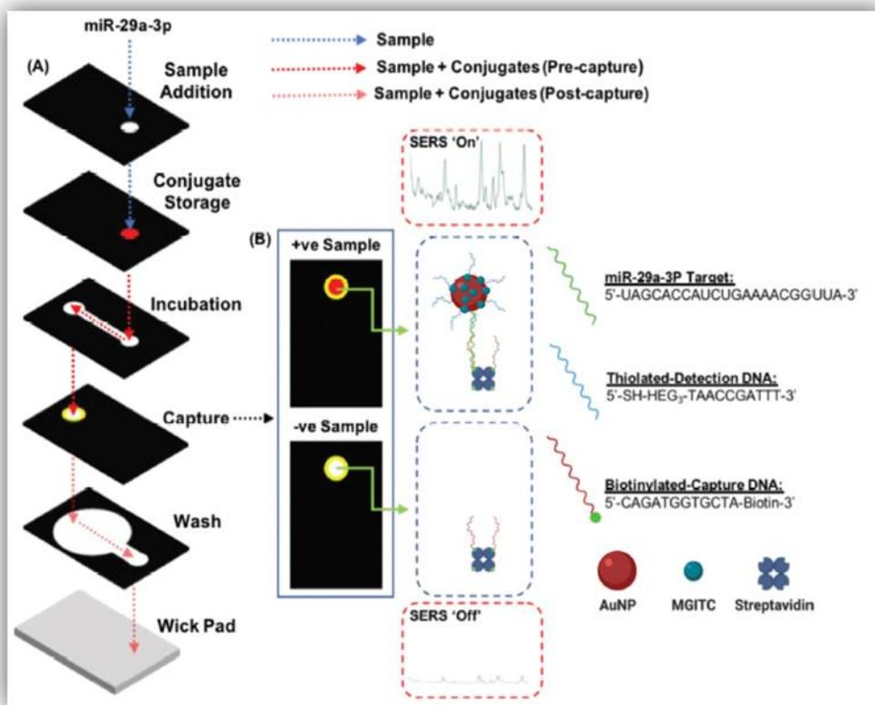
**Figure 7. Schematic of a microfluidic paper-based diagnostic platform for the detection of miR-29a using colorimetric and SERS analysis [78].**
