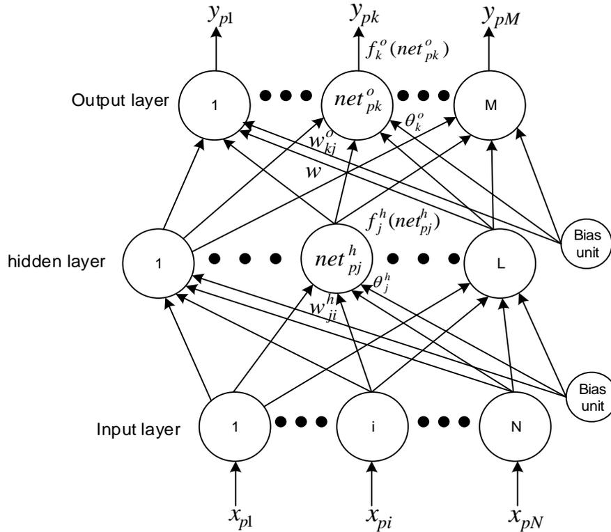
Fig. 2. Architecture of feed-forward neural network structure
