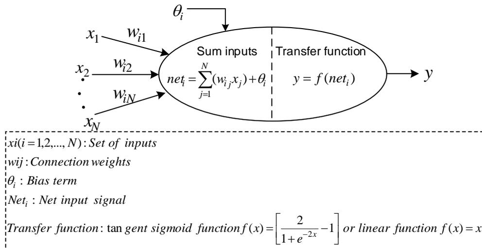
Fig. 3. Structure of a typical artificial neuron
