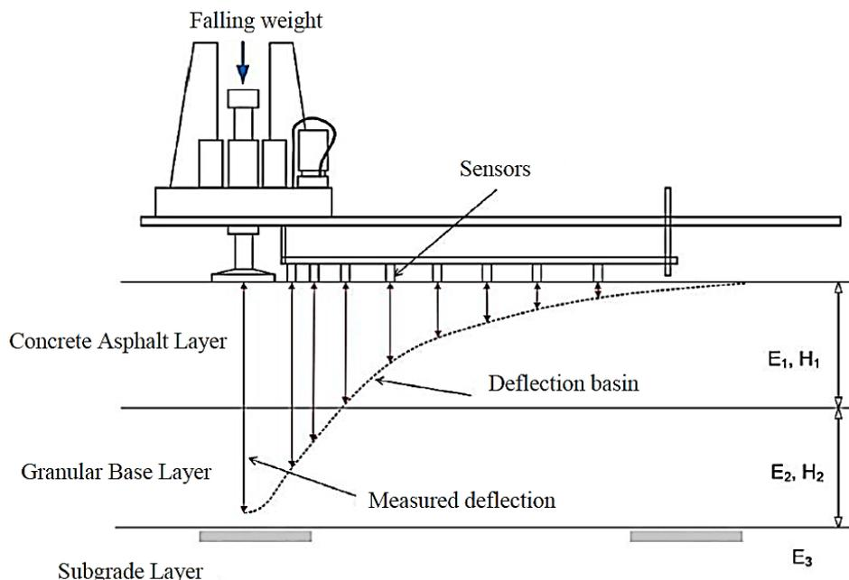
Fig. 1. Schematic image of the FWD and measuring the deflection basin for a flexible pavement
