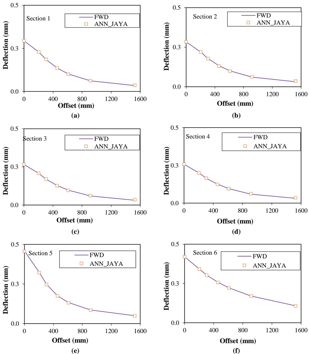
**Fig. 11.** Deflection basins calculated based on the JayaBack backcalculated moduli and ones measured by the FWD device; a) Section 1; b) Section 2; c) Section 3; d) Section 4; e) Section 5; and f) Section 6
