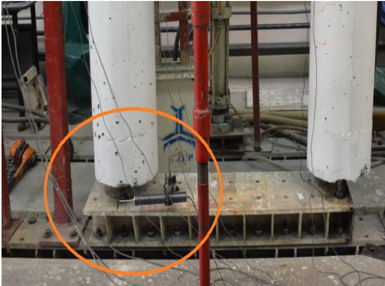
Fig. 6. Possible slip control of the specimen relative to the steel beam
