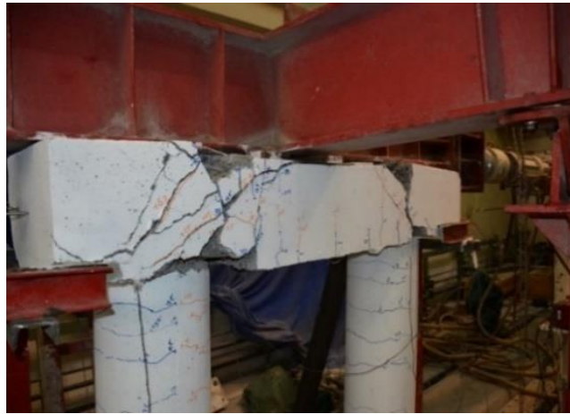
Fig. 14. Ultimate damage mechanism for SP-80
