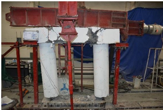
Fig. 15. Ultimate damage mechanism for SP-90
