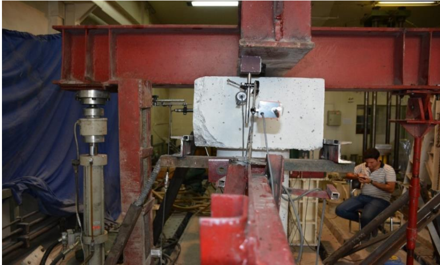
Fig. 8. Applying gravity load
