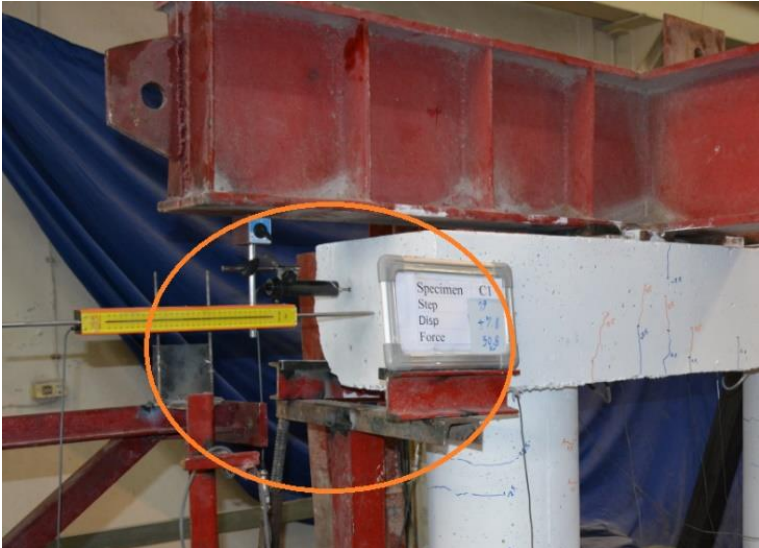
Fig. 5. Displacement control of the end of the cap beam relative to the rigid floor
