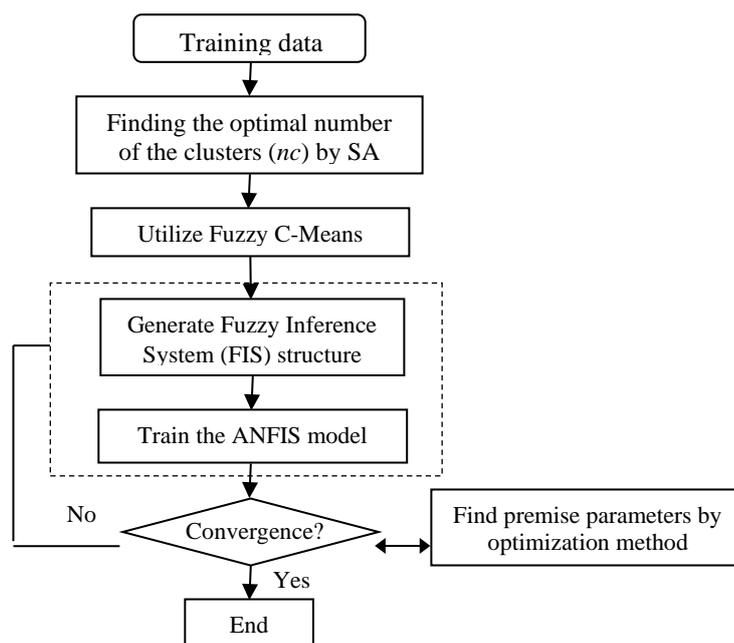
Fig. 3. Flowchart of the proposed ANFIS method with optimization methods
