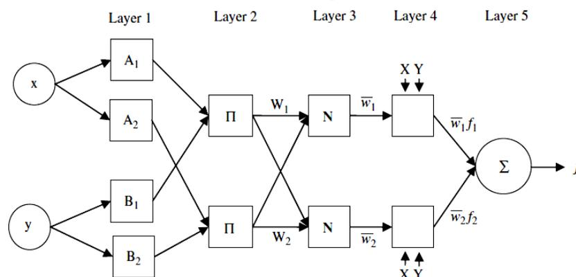
Fig. 2. The architecture of the ANFIS model
