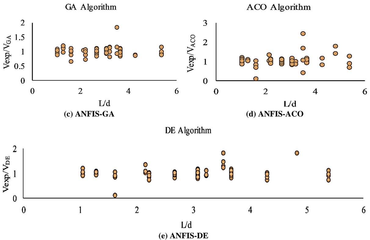
**Fig. 5.** The changes of the ratio of the experimental shear strength to the predicted shear strength in term of  $L/d$  parameter
