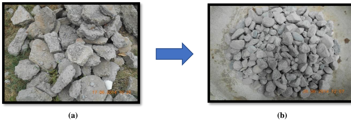
Fig. 1. a and b) Recycled concrete aggregates processed from demolished concrete waste
