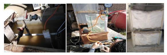
Fig 5. Our membrane operates within the MBR system of the Dairy factory of the College of Agriculture.
