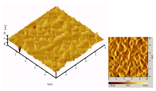
Fig 11. AFM images of composite flat sheet membrane (CFSM-2)
