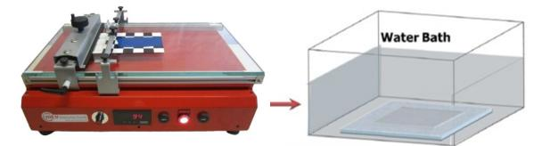
Fig 3. Phase inversion process for composite membranes fabrication using the motorized film applicator CX-4 (Germany)
