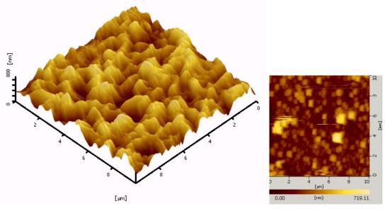
Fig 10. AFM images of composite flat sheet membrane (CFSM-1)
