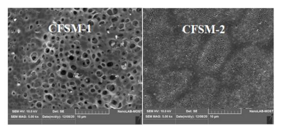
Fig 7. SEM images of composite flat sheet membranes with and without the nanomaterials.
