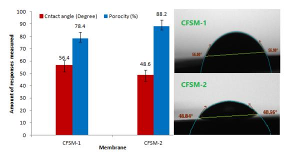
Fig 12. Static water contact angle and porosity of the composite membranes
