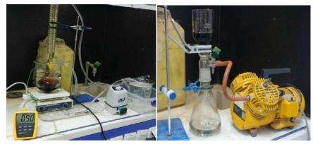
Fig 2. Preparation of the oxidized MWCNTs.
