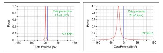
Fig 15. Zeta potential data for fabricated membranes (CFSM-1 and CFSM-2).
