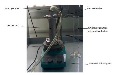
Fig 4. Photograph of the dead-end filtration cell (STERLITECH HP4750)
