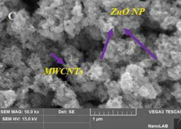
Fig 6. SEM imeges: (a) raw MWCNTs (b) oxidized MWCNTsand (c) OMWCNTs/ZnO/ AG
