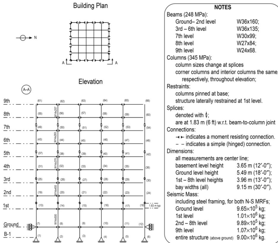
Fig. 6. 9-Story benchmark building N-S MRF (Ohtori et al., 2004)
