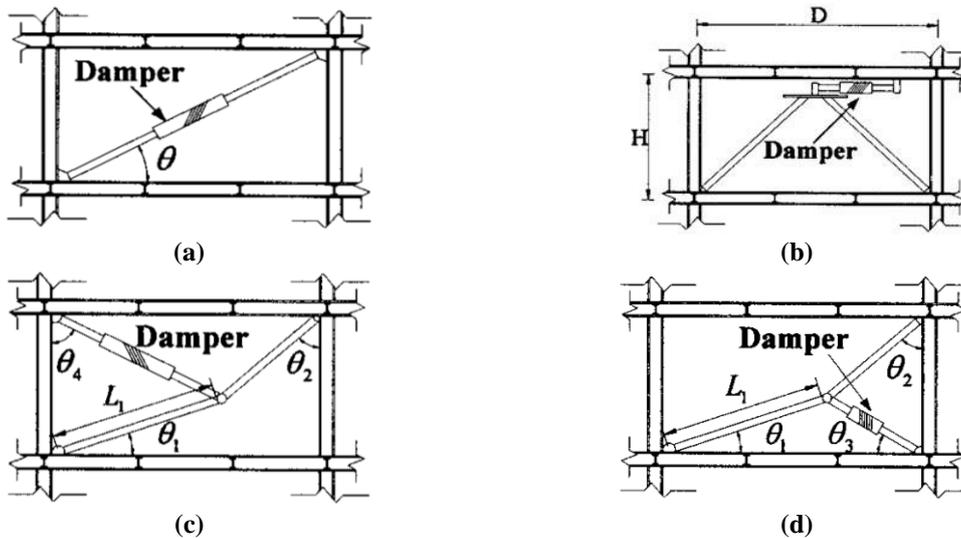
**Fig. 1.** Installation schemes of viscous dampers: a) Diagonal brace; b) Chevron; c) Upper toggle brace; and d) Lower toggle brace
