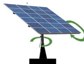
Figure 3. Two-axis solar tracker [43]
