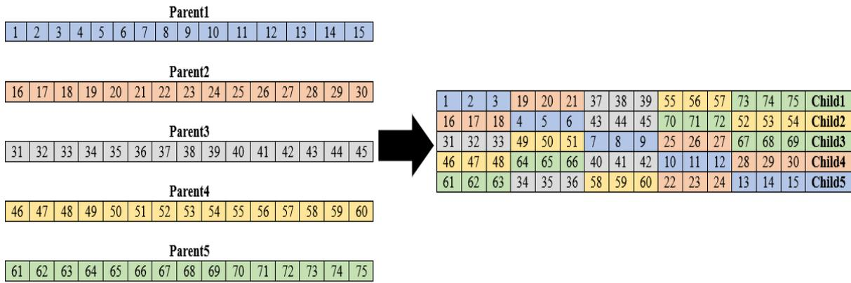
Figure 5. Multi-Parent cross-over in MPNSGA-II algorithm (five parent)
