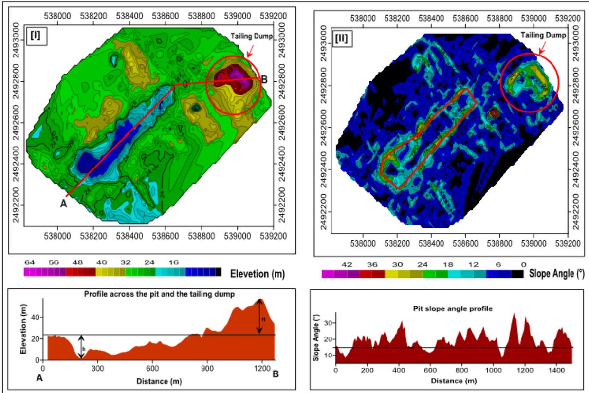
Fig . 3. The pit terrain characteristics, (I) is the topographic map of the pit and its surroundings and (II) depicts the terrain slope angle
