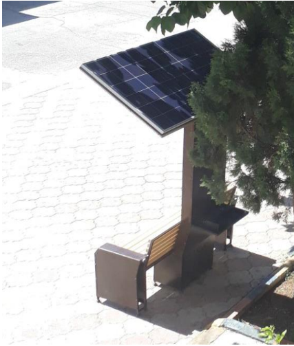
Figure 6. The panel that used in the solar bench
