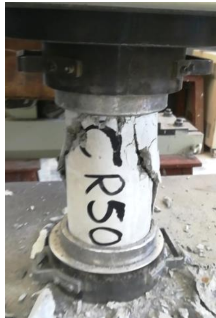
(b) Damage/Crack pattern in CR50
