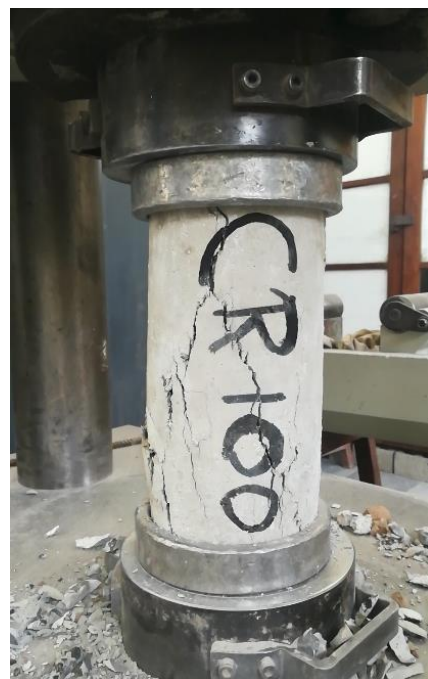
(b) Damage/Crack pattern in CR100
