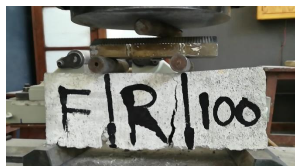
(b) Damage/Crack pattern in FR100
