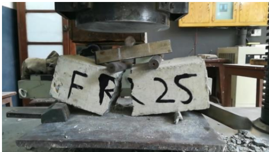
(a) Damage/Crack pattern in FR25
