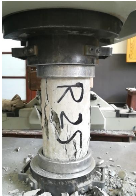
(a) Damage/Crack pattern in CR25
