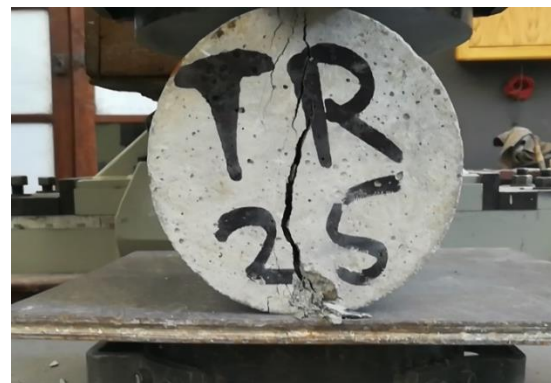
(b) Damage/Crack pattern in TR25
