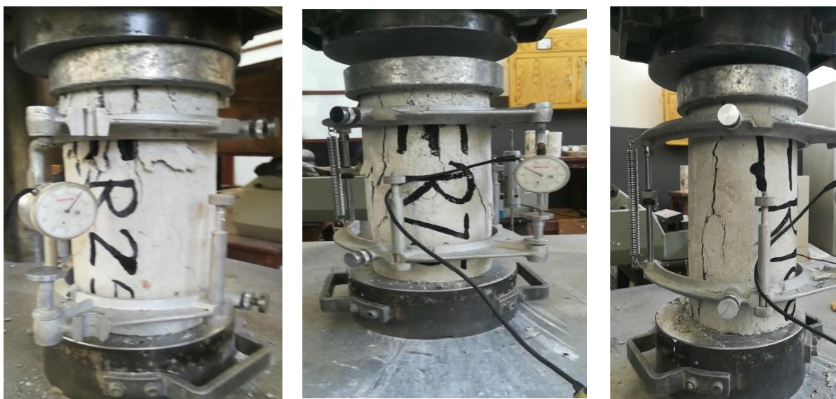
(c) Damage/Crack pattern in R100
