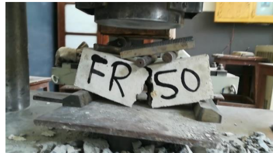
(b) Damage/Crack pattern in FR50
