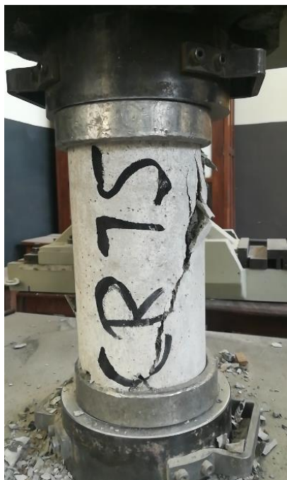
(a) Damage/Crack pattern in CR75
