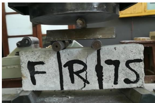
(a) Damage/Crack pattern in FR75
