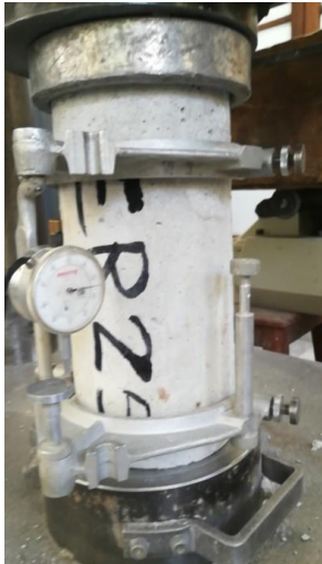
Fig. 6. Compression test in UTM
