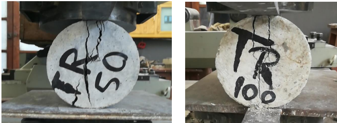
(a) Damage/Crack pattern in TR50
