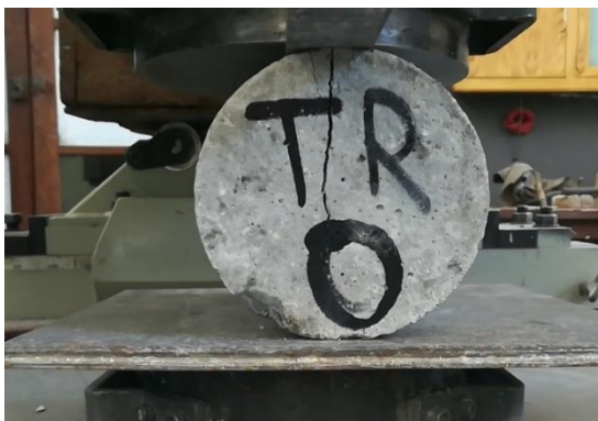
(a) Damage/Crack pattern in TR0
