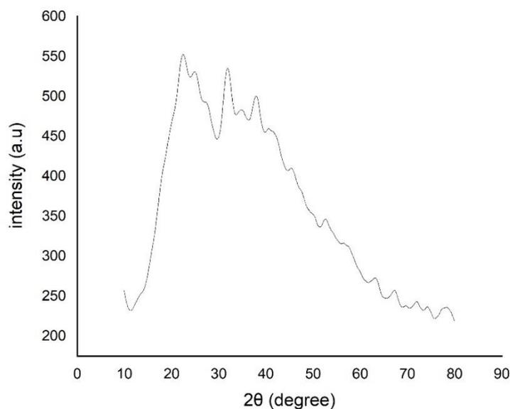
**Figure 2.** X-ray diffraction (XRD) patterns of p(AM-co-AA)
