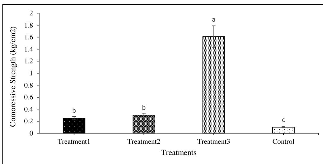
**Figure 5.** Effect of mulch types on compressive strength of sand samples
