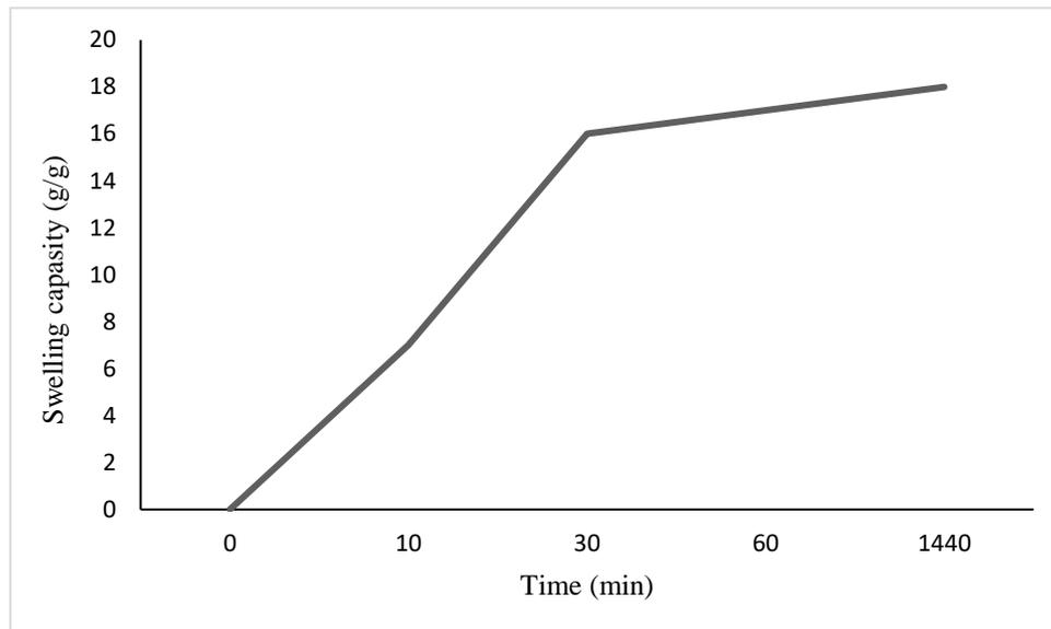
**Figure 4.** Swelling capacity curves of the prepared hydrogels in distilled water
