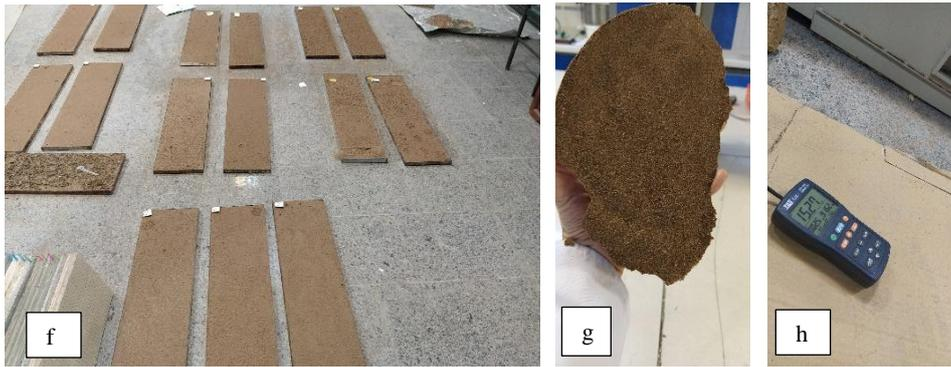
**Figure 9.** a: hand core penetrometer b: geo Tor vane shear tester c: wind tunnel d: abrasion tester e: steel bar for impact resistance f: metal trays of treatments g: sand attachment with mulch utilization h: maximum wind created by wind tunnel
