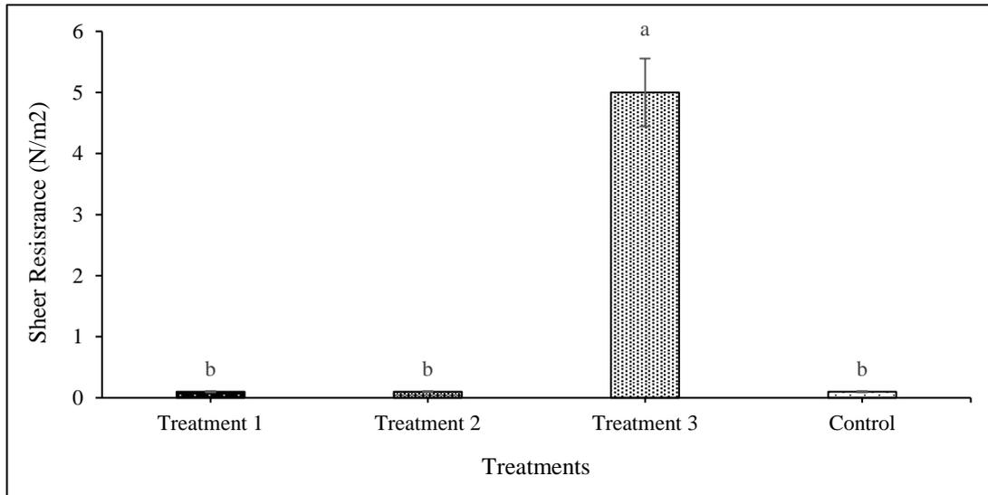
**Figure 6.** Effect of mulch types on shear strength of sand samples
