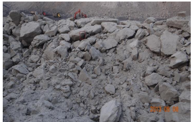
Figure 26. Fragmentation obtained using the pilot holes and pocket charges at the 4 th Bench, Quarry No. 2
