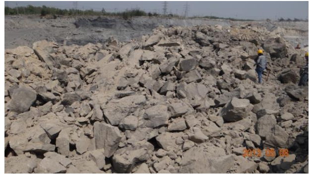
Figure 25. Fragmentation obtained using the pilot holes and pocket charges at the 1 st Bench (Matin-Di area).
