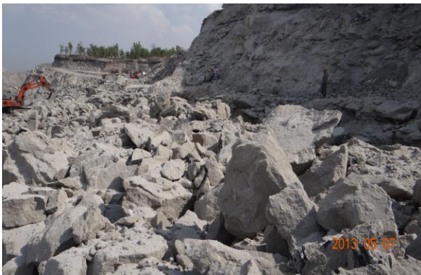
Figure 22. Oversize boulders generated from the top portion of the holes in the trial blast conducted with the decked charge at the 3 rd Bench coal-touch (Matin-Di area).
