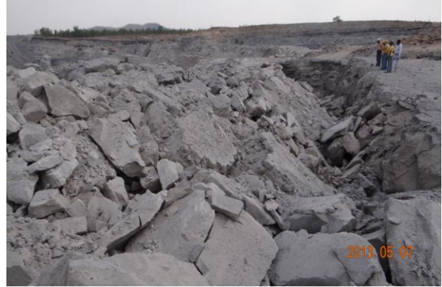
Figure 24. Good cut with minimum backbreak obtained with the decked charge.
