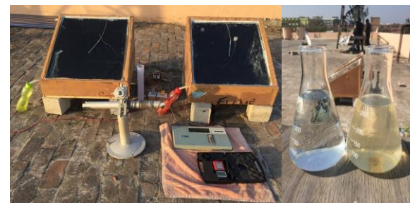
Figure 4.a) Photograph of modified still and conventional still; b) photograph of freshwater and brackish feed water
