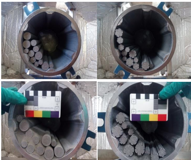
Fig. 5. Dispersing of simple rods and grooved rods on the mill liner surface.
