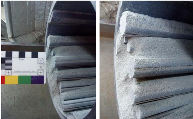
Fig. 4. The spoon action of grooved grinding rods in rod mill.
