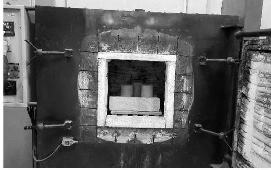
**Fig. 3** Electric heating furnace
