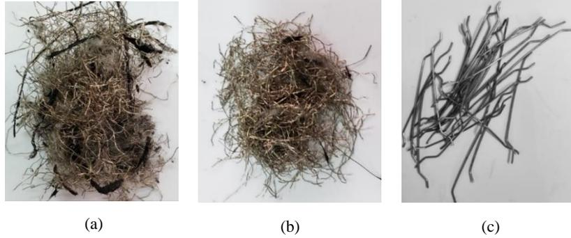
**Fig. 1** Steel fibers used: (a) RSFI, (b) CRSF, and (c) ISF
