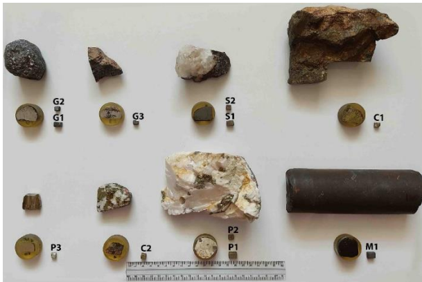
Fig. 2. 11 samples are separated from the metal ores illustrated in the Figure and used in bipolar electrochemistry experiments. S1 and S2: sphalerite, M1: magnetite, P1 to P3: pyrite, C1 and C2: chalcopyrite, and G1 to G3: galena. The characteristics of the samples are reported in Table 1. The polished section of the samples was prepared and studied (see, Fig. 3).
