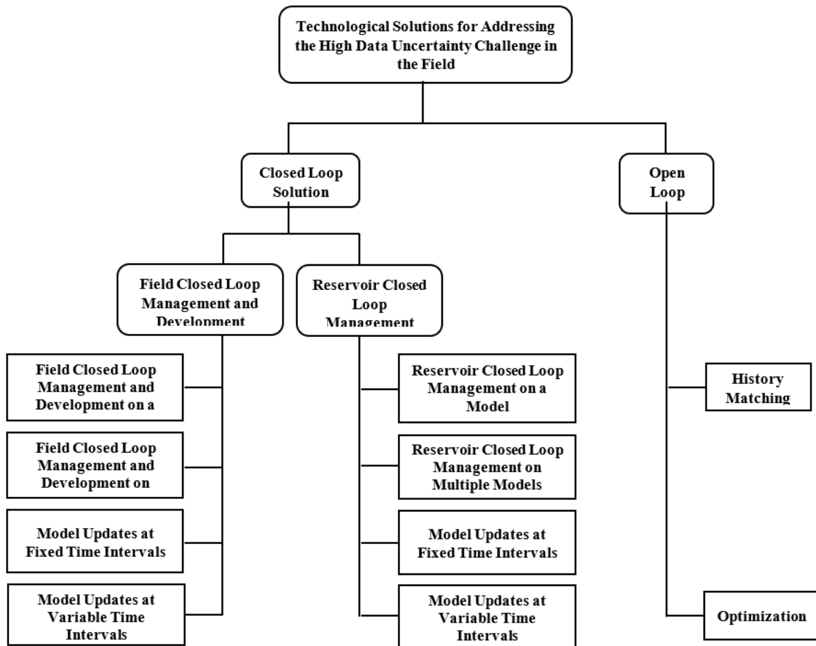
Figure 7) Tree of technological solutions to address the challenge of high uncertainty in field data.
