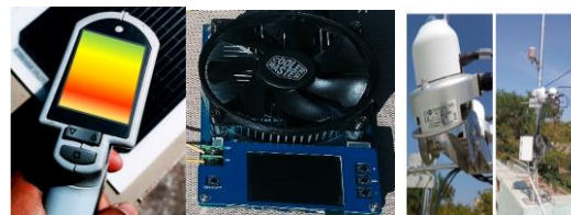
Figure 6. (a) fluke thermal camera (b) Electronic load circuit (c) Pyranometer
