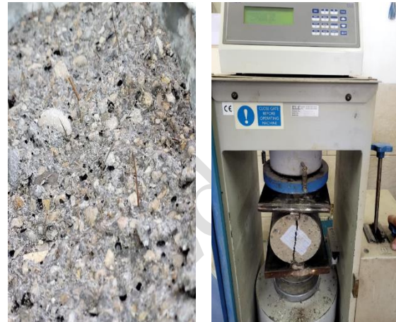
Fig. 8. Failure of the cylindrical test piece with the Brazilian device and the test piece broken with palm fibers
