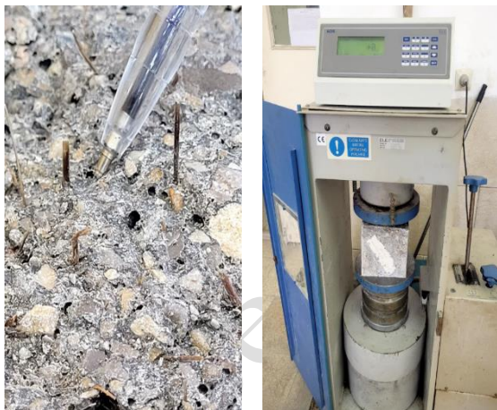
Fig. 7. The failure of the cube specimen with the compressive strength device and the specimen broken with palm fibers
