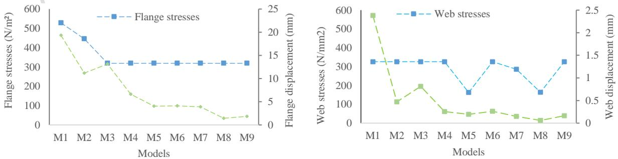
Fig. 13. Stresses and displacement at (a) column flange and (b) column web of the numerical models.
