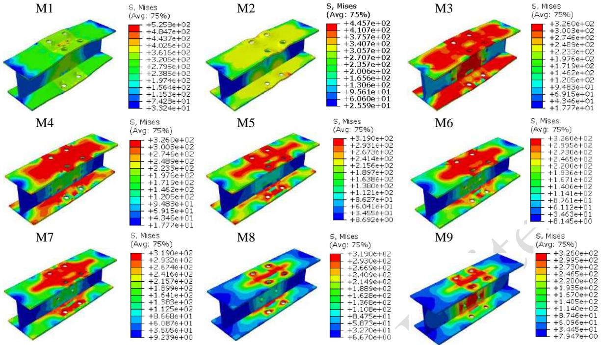
Fig. 11. Column flange stress of the numerical models
