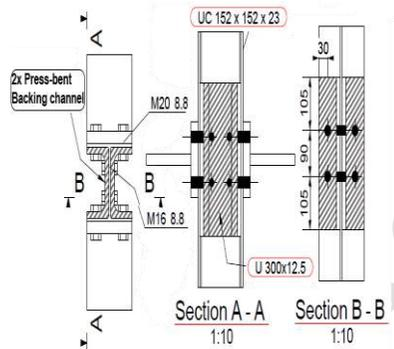
g) T7 Test (300x12.5 backing channel bolted to col.web)
