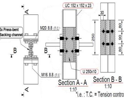
h) T8 Test (250x10 backing channel bolted (HA bolts) to col.web)
