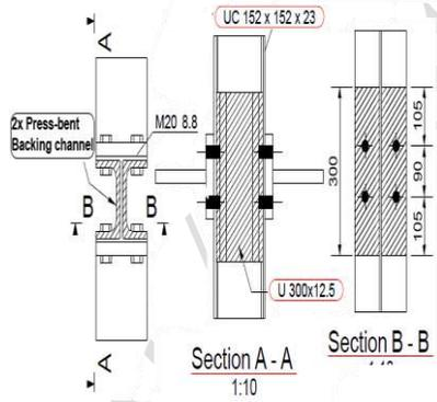
e) T5 Test (300x12.5 backing channel)
