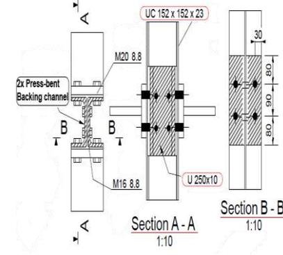
f) T6 Test (250x10 backing channel bolted to col.web)
