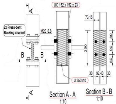
d) T4 Test (250x10 backing channel)
