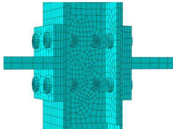
**Fig. 4.** Finite element mesh of the T-stub connections.
