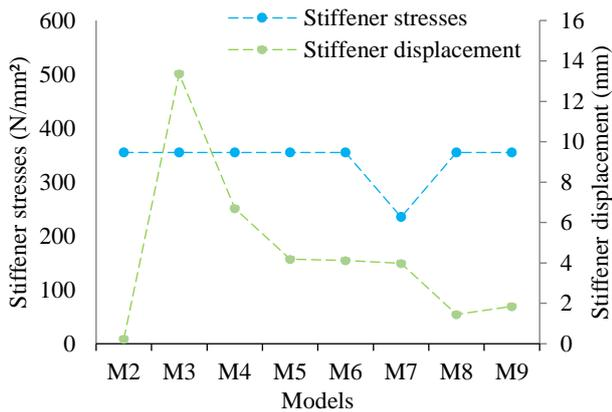
Fig. 16. Stiffener stresses and displacement of the numerical models
