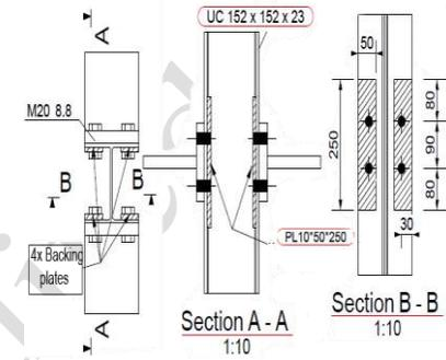
c) T3 Test (250x10 backing plates)
