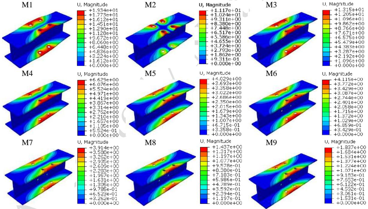
Fig. 12. Column flange displacement of the numerical models
