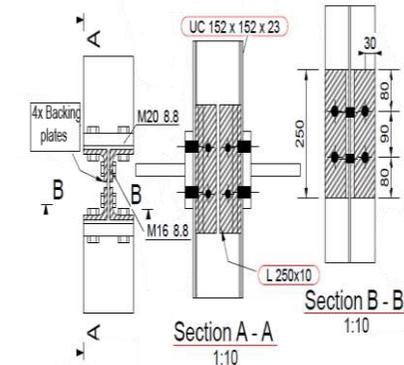
i) T9 Test (250x10 backing angles bolted to col.web)
