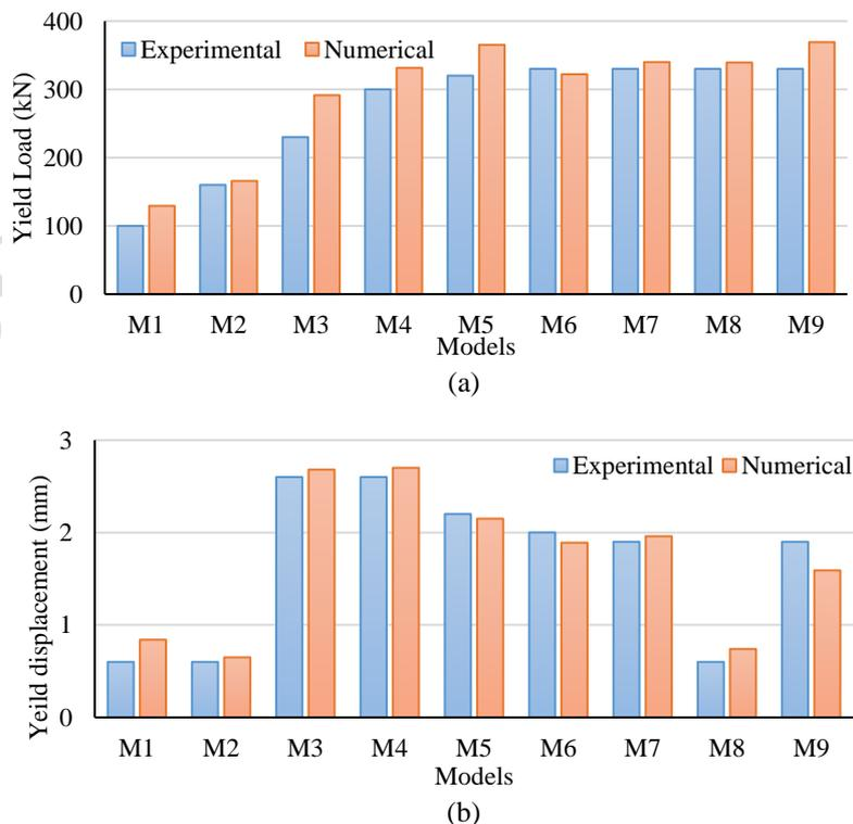
**Fig. 8.** Comparison between numerical and experimental results for (a) yield load, and (b) yield displacement.
