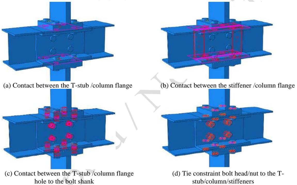
**Fig. 5.** Contact interactions and ties constraint of the models.
