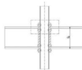
Fig. 1. (a) Extended end-plate connection and (b) its T-stub idealization
