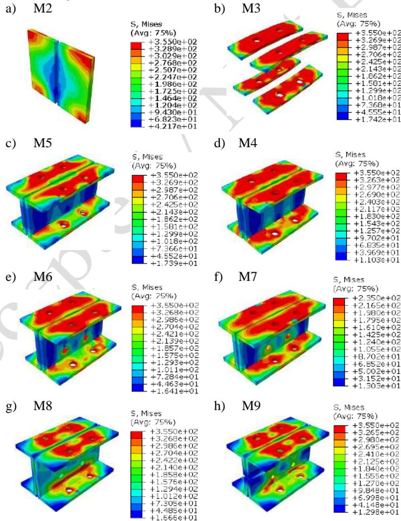
Fig. 14. Von Mises stresses of the stiffeners
