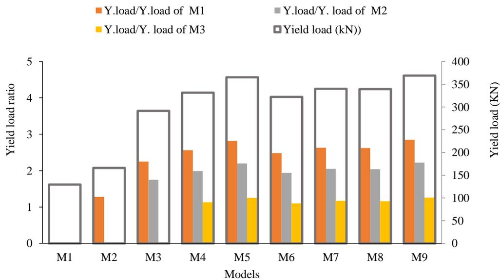
Fig. 10. Comparison on load capacity at 0.003 rads between the nine models.
