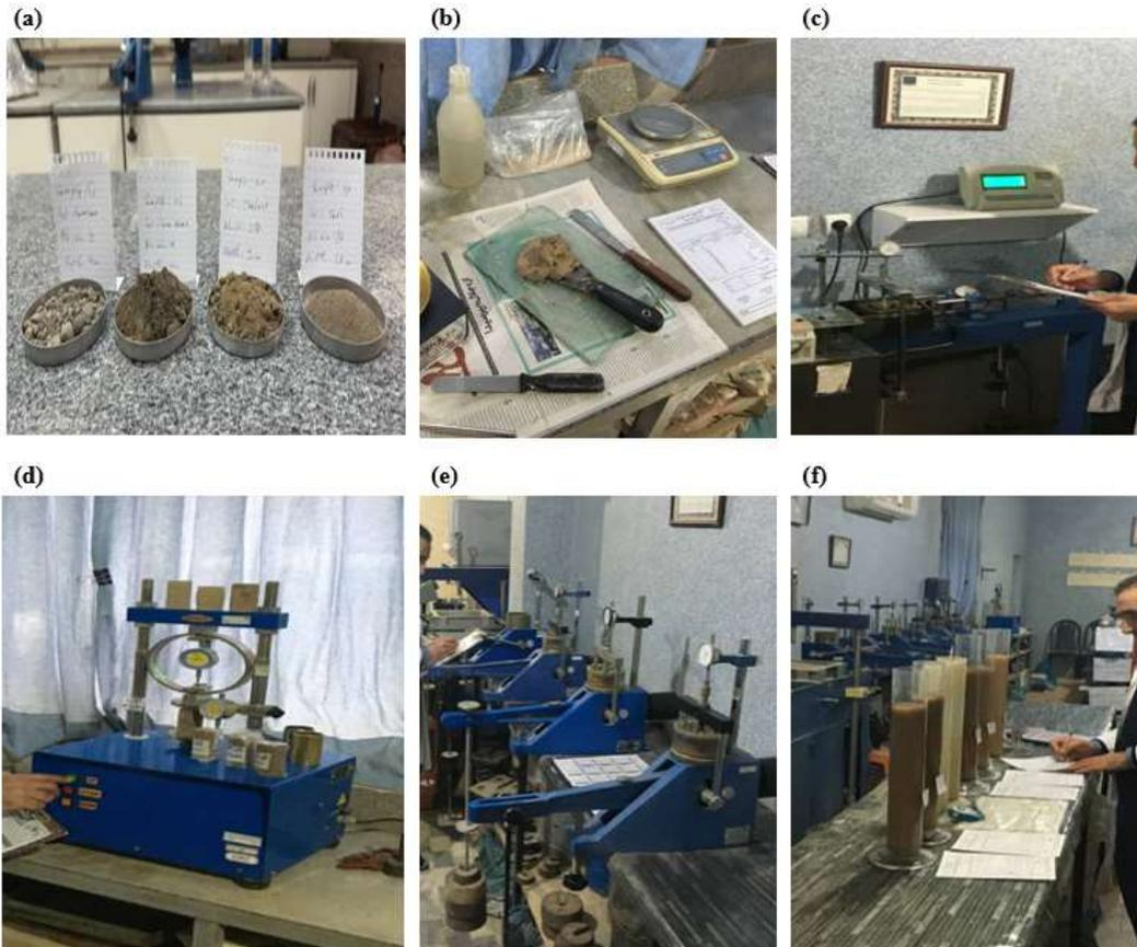
**Figure 6.** (a) an example of different soil types, (b) Atterberg limit tests procedure, (c) direct shear test instrument, (d) unconfined uniaxial compressive test, (e) consolidation test procedure, and (f) hydrometer test procedure
